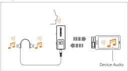
Two way transmission of audio between transmitter and receiver, audio can be monitored in transmitter and receiver
